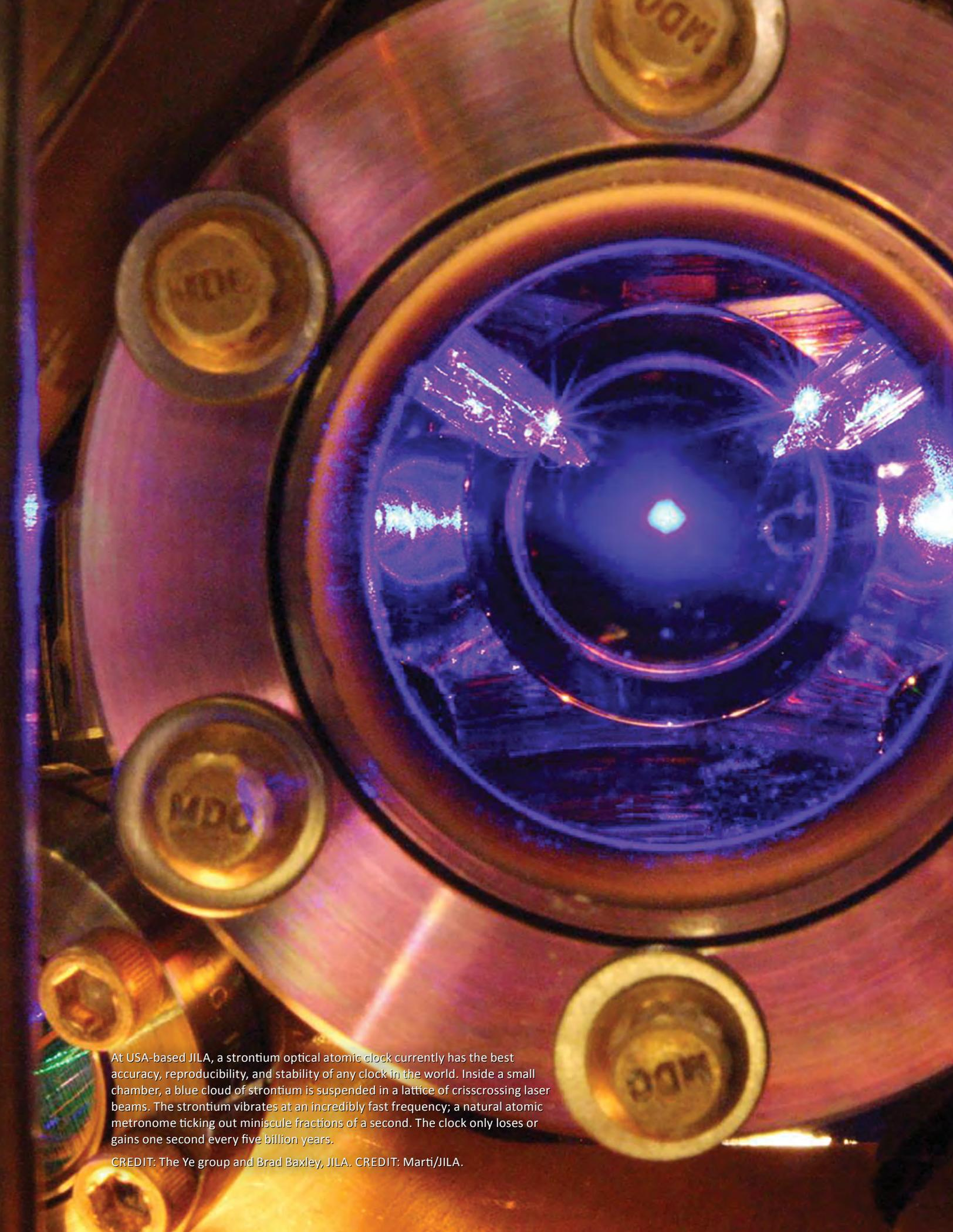
At USA-based JILA, a strontium optical atomic clock currently has the best accuracy, reproducibility, and stability of any clock in the world. Inside a small chamber, a blue cloud of strontium is suspended in a lattice of crisscrossing laser beams. The strontium vibrates at an incredibly fast frequency; a natural atomic metronome ticking out minuscule fractions of a second. The clock only loses or gains one second every five billion years.
