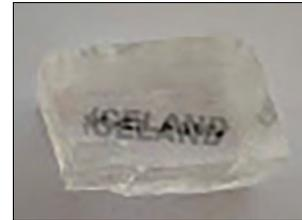
The little crystal, Iceland spar, baffled Isaac Newton and others by splitting light into two beams. The spar and its anomalies ultimately led to the downfall of Newton's particle theory of light. CREDIT: Bruce Watson.
